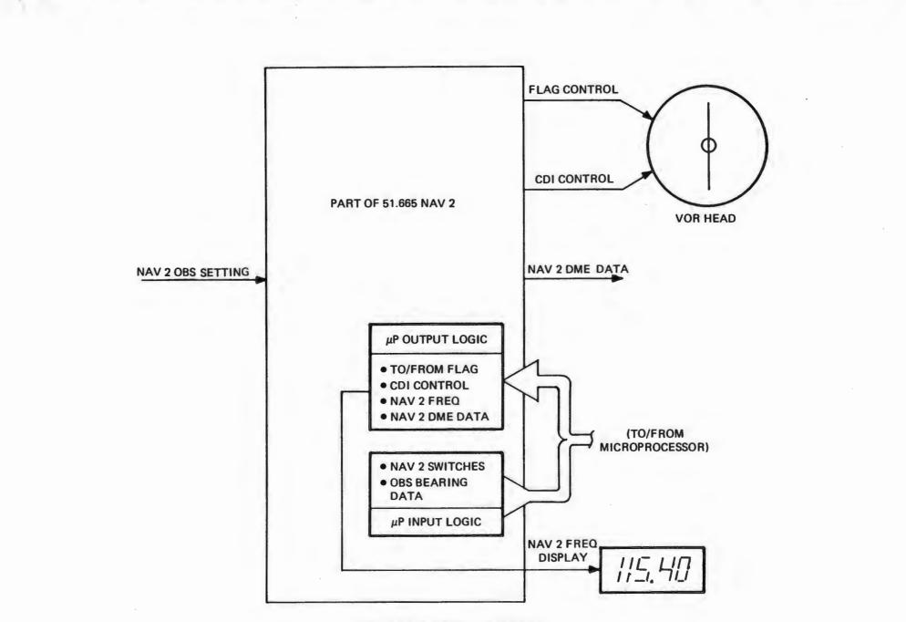
Figure 2.5 Block Diagram of NAV 2 Major Functions
