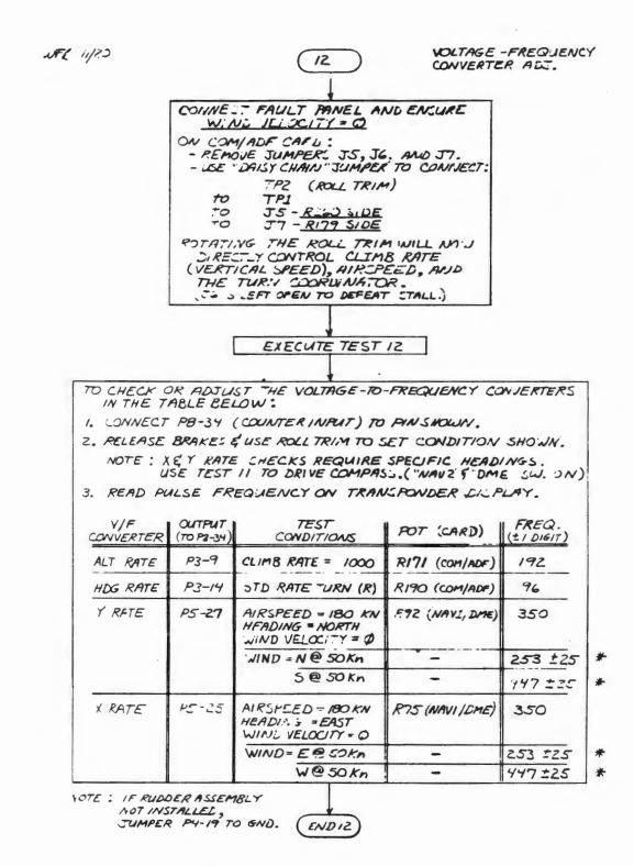
\* THESE ARE CHECKS, NOT ADJUSTMENTS. THE CIRCUITRY IS ON THE FAULT PANEL & NAVI / DME.
