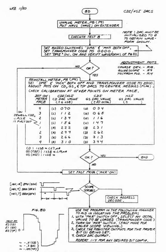
DAC WAVEFORMS WITH METER UNPLUGGED. ALL & STEPS CAN BE SEEN (USE HP ISON - PUT . OI , OT ACROSS INPUT TO FILTER NOISE)
