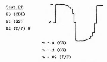
DAC waveforms with meter unplugged. All 8 steps can be seen (use HP 130A- put .01µf across to filter noise)
