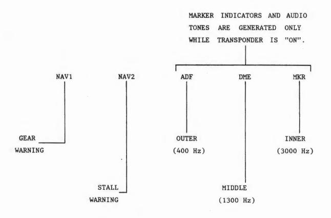
\*Operate HI/LO test switch and hear a change in volume.
