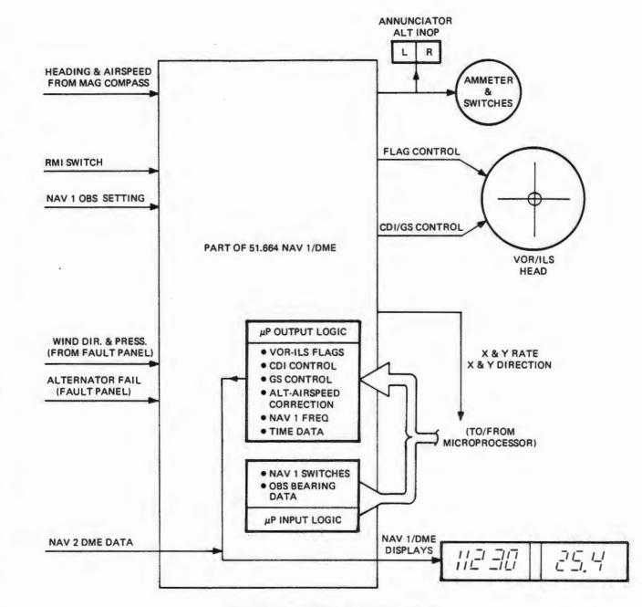
Figure 2.4 Block Diagram of NAV 1/DME Major Functions
